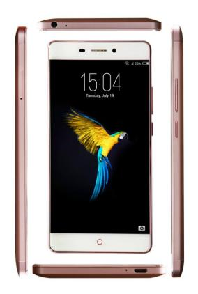
On top of this Mango 3D are the light sensor, earphone and video camera. Downside is a small circle as for HOME button. On each side of the HOME button, there are MENU and RETURN buttons. Those two buttons light on only when it is under operation. Back cover is metal material with curve design. It is quite comfortable holding in hand. On top of the back cover, there are rear camera, the finger printer identifier, as well as loud speaker. Colored with rose gold.
